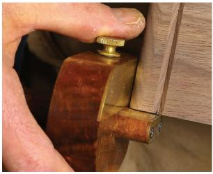
**Transfer the V-groove line.** Use a marking gauge resting on the end of the board with the blade just hitting the bottom of the V-groove. Transfer that line to the other side of the knuckle stock.
