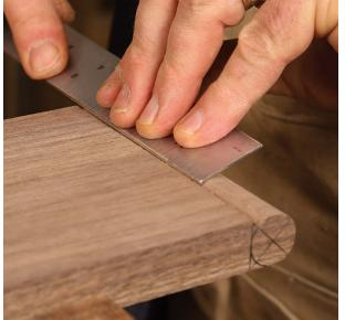
Refine the round. Use a chisel to complete the curve of the barrel and smooth it into the V-groove. Latta backs a metal ruler with sandpaper to smooth the curve even more.
