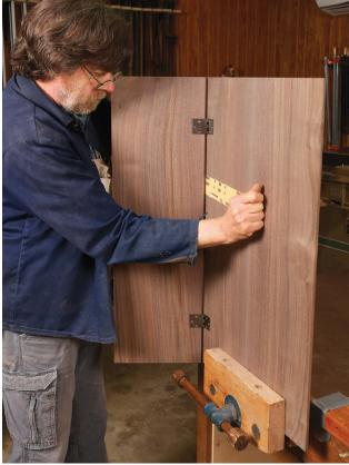
**Install the hinges.** Once the hinge mortises are cut, install all the hinges, and test the fit. If you need to, shimmy a strip of sandpaper backed with packing tape in the joint and slide it back and forth along the length of the joint to tweak the fit.
