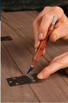
**Transfer the hinge placement.** With the hinges set in place in the top, set the top and the leaf next to each other (with a commercial veneer between them as a spacer), and clamp them in place. Score the outline of the hinges onto the leaf, and use a trim router to waste out the mortise and a chisel to clean to your line.
