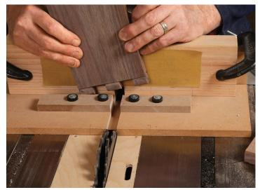
**Excavate between the knuckles.** Using a carriage to hold the parts, raise the dado head to the midpoint of the V-cut. First make a cut in the middle of the knuckle and then slide left or right, aligning directly to the score marks. The carriage is screwed to two miter gauges.
