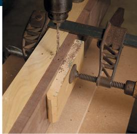
Flip and drill through. After drilling the first half of the knuckle joint, remove the workpiece, insert a length of steel rod in the registration hole, flip the knuckle board over, and seat the just-drilled hole on the registration pin. Make sure the same face of the board is against the fence, and drill through the knuckle into the first hole. Tap in a pin whose length is just less than the full width of the apron. The hinge should swing smoothly but stiffly.
