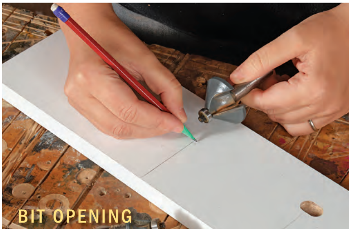
The opening should fit your biggest bits. You will most likely use this auxiliary fence with large router bits, so use your largest bits, both in width and height, as a guide for laying out this opening.
