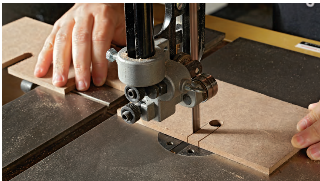
Finish the spacers at the bandsaw. After drilling the bolt holes, turn them into slots at the bandsaw. The slots will allow you to slide the spacer over the bolts to insert or remove it. Having drilled out the corners of the bit opening, Hannah bandsaws it to final shape too.
