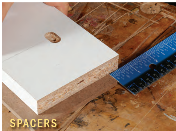
Drill bolt holes on spacers lower than on the auxiliary fence. Making the holes lower will leave a slight gap underneath a spacer when it is installed, so it's easier to remove. Use the drill bit you used on the auxiliary fence to mark the spacer (right).
