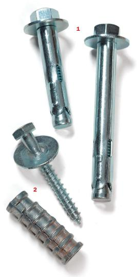
When you want to attach with screws or lag screws, use lead sleeve anchors. These old-style Everbilt soft lead lag sleeves (2) are studded with projections and built in two loosely connected halves, allowing them to expand and shift in shape to conform to a predrilled hole when the screw is driven home.
