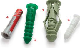
The Cobra Triple Grip (1), intended for all wall types, is rated for 46–61 lb. in drywall, 200–225 lb. in masonry; Everbilt Ribbed Plastic Anchors (2 and 3), which come in kits of assorted sizes, are rated for 20– 25 lb. in drywall, 155–435 lb. in concrete; Duo Power plastic anchors (4) elbow open and are rated for 45 lb.
